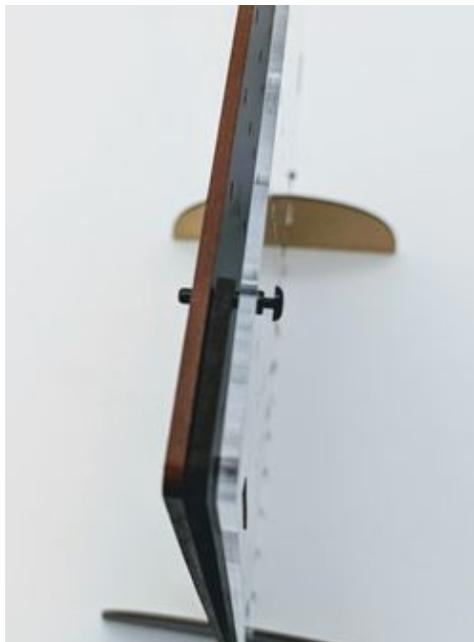
Insert the pop rivets (shown above) or M3 screws/acorn nuts through each of the 107 holes between the wooden base and the cover. The acorn nuts will tighten to a fixed position on the screws, which prevents too much force being applied to the acrylic cover. If you use regular screws and nuts, be sure not to over tighten them. The acrylic should not bend anywhere.
