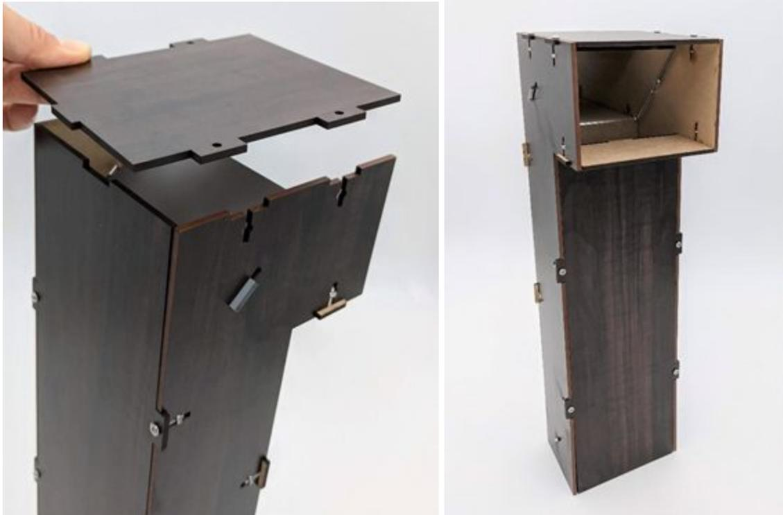
Place the remaining wooden piece at the top of the periscope. The tab of the topmost piece slots into the notch at the back of the periscope as shown. Fasten the top to the sides with screws and nuts.
