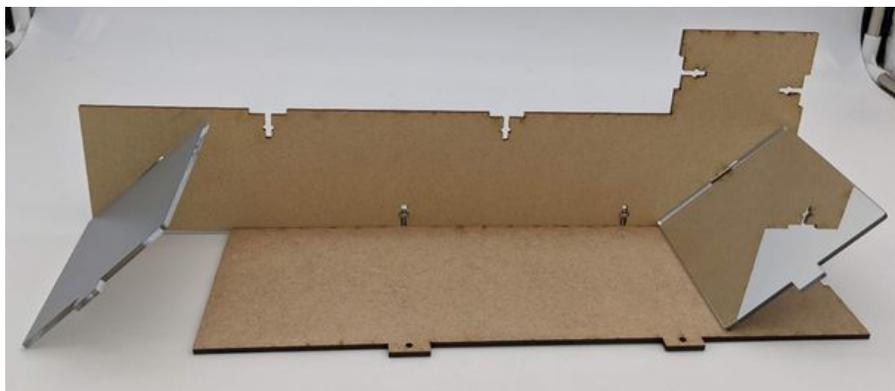
We'll prepare to attach the other side piece of the periscope, but before securing it with screws and nuts, place the two pieces of mirrored acrylic between the angled slots in the periscope sides. Be sure that the reflective sides of the acrylic face towards each other as shown in the picture.
