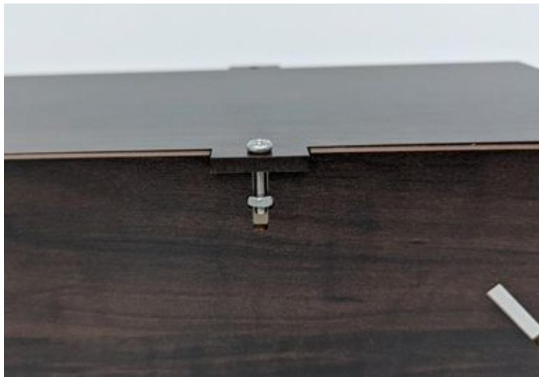
Slide an M3 nut into the cross portion of one of the small “t” shaped notches in the side, and insert a 14mm M3 screw through the hole in the tab until it reaches the nut. Twist the screw with your fingers until it engages with the nut, then continue to tighten it with a screwdriver until it secures the two wood pieces together. Do the same for the other matching slot and tab in the two pieces.
