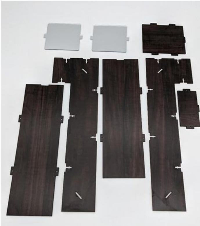
Cut the reflectors from the mirrored acrylic using the vector file “PeriscopeMirrors.svg”. Using a laser cutter with a mirror can be dangerous if the laser reflects off of the mirrored surface, so be sure that the mirrored surface of the acrylic is facing downwards when being cut, or that it is covered with protective paper.
